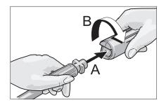
**Step 2**Insert the spray wand of your choice into the trigger gun. Press in against the spring tension (A) and twist into the locked position (B).
